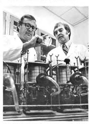
THE ANDERSON AIR SAMPLER separates dust by particle size and deposits the particles on glass disc. Charles and Lial examine one of the discs before insertion into the sampler; later the deposits will be analyzed to determine if toxic dusts are present.
